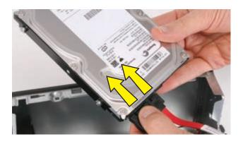
4 Place the drive so the guide screws fit into the guide screw slots. The drive manufacturer's label should be visible when the drive is in place.
